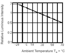
Ambient Temperature  $T_a = {}^{\circ}C$ Luminous Intensity vs. Ambient Temperature
